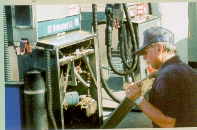
An employee of the Department of Weights and Measures checks a gasoline pump for accuracy.
